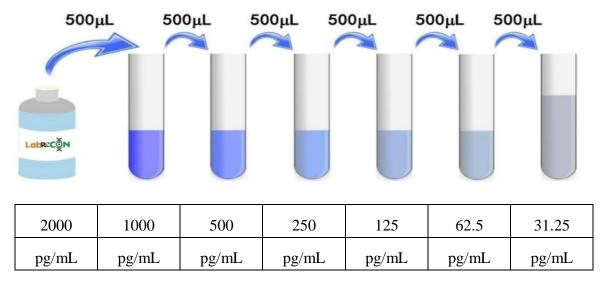
$5.1 \times$  Biotinylated Detection Ab and  $1 \times$  HRP Conjugate Working Solution - Briefly spin or centrifuge the stock Biotinylated Detection Ab and HRP Conjugate before use. Dilute them to the working concentration 100 folds with Biotinylated Detection Ab Diluent and HRP Diluent, respectively. For example,  $10 \,\mu$ L of HRP Conjugate with 990  $\mu$ L of HRP Diluent.
