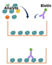
1、Add 50µL standard or sample to the wells, immediately add 50µL Biotinylated Detection Ab working solution to each well. Incubate for 30 min at 37°C
