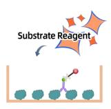
4、Add 100µL Substrate Reagent. Incubate for 15 min at 37℃
