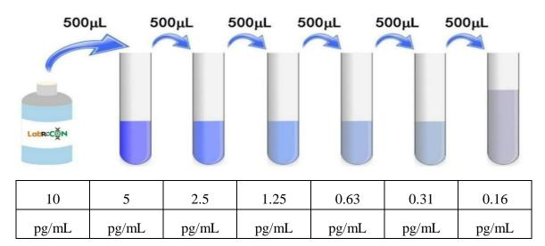
$5.1 \times$  Biotinylated Detection Ab and  $1 \times$  HRP Conjugate Working Solution - Briefly spin or centrifuge the stock Biotinylated Detection Ab and HRP Conjugate before use. Dilute them to the working concentration 100 folds with Biotinylated Detection Ab Diluent and HRP Diluent, respectively. For example,  $10 \,\mu$ L of HRP Conjugate with 990  $\mu$ L of HRP Diluent.
