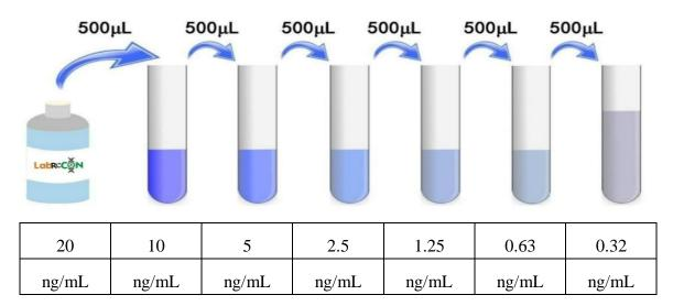
5.1× Biotinylated Detection Ab and 1× HRP Conjugate Working Solution - Briefly spin or centrifuge the stock Biotinylated Detection Ab and HRP Conjugate before use. Dilute them to the working concentration 100 folds with Biotinylated Detection Ab Diluent and HRP Diluent, respectively. For example, 10 μL of HRP Conjugate with 990 μL of HRP Diluent.
